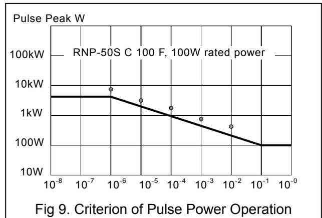
Fig 9. Criterion of Pulse Power Operation
