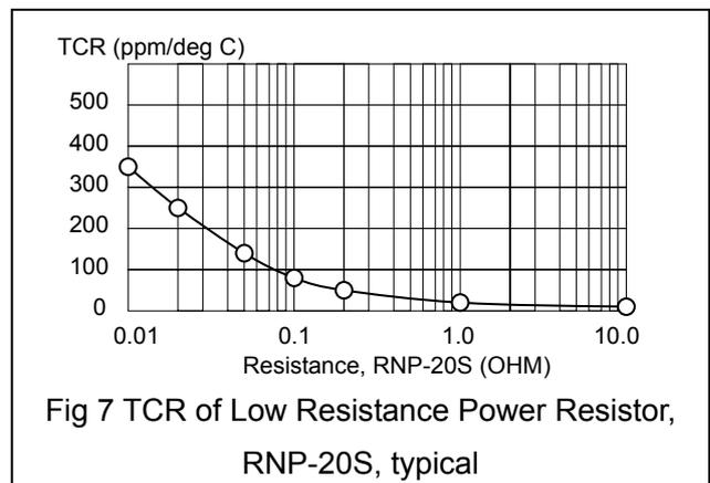
Fig 7 TCR of Low Resistance Power Resistor, RNP-20S, typical
