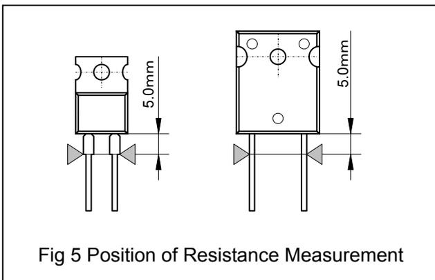
Fig 5 Position of Resistance Measurement
