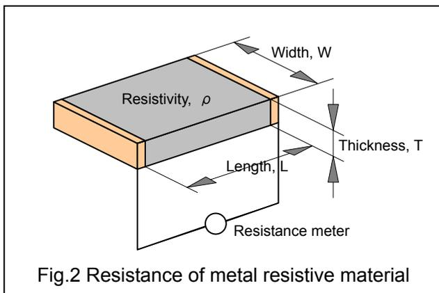
By the calculation of resistance of the metal which is cut 10mm square with 0.1mm thickness, a resistance between the both side points of the metal is calculated as Table1.
