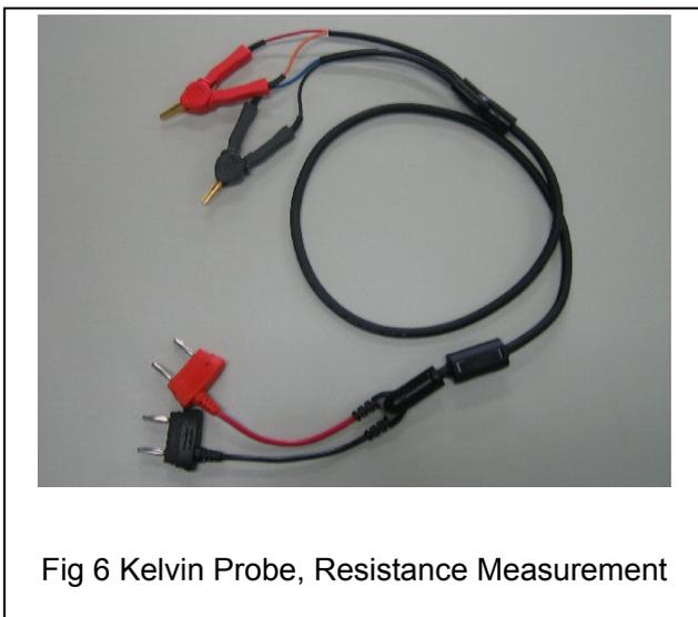
Fig 6 Kelvin Probe, Resistance Measurement
