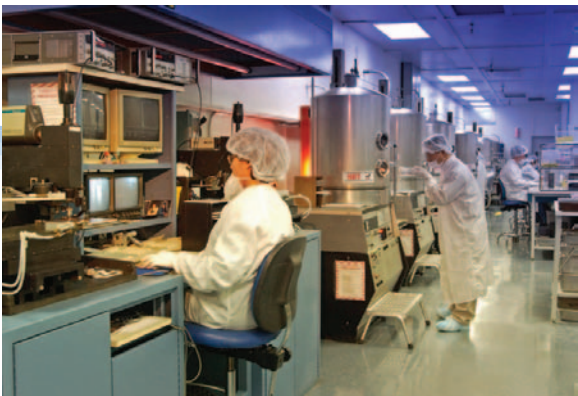
Both laser trimming and wafer backplating allow Statek to achieve tight frequency tolerance of crystals while in wafer form.
