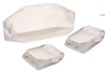
Statek's process begins with ultra-pure, synthetically-grown Alpha quartz or swept quartz for radiation-sensitive applications.
