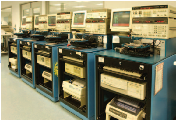
Statek uses automated work stations to measure accurately device parameters from wafer probe through final test.
