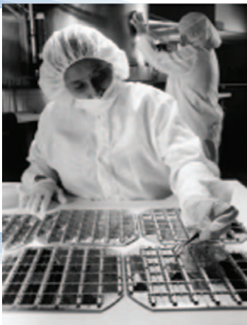
Wafers are processed into arrays of various quartz resonators.
