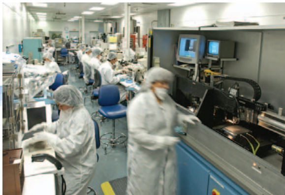
Custom built automated equipment precisely assembles crystal resonators.
