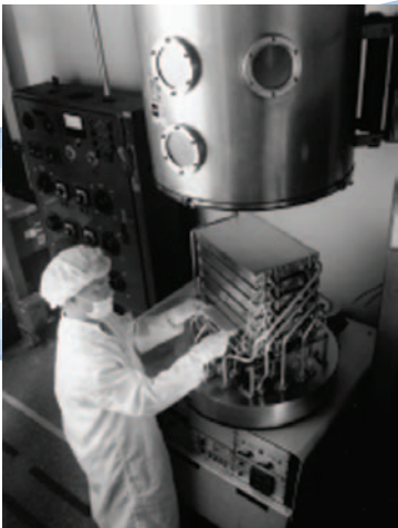
The ability to seal parts with a glass lid allows Statek to adjust frequency after assembly to produce extremely accurate and stable products.
