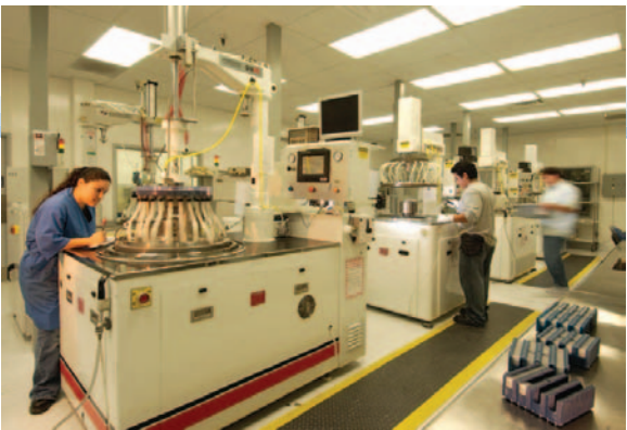
Quartz bars are lumbered, sliced and lapped. Wafers for special applications are further polished to an optical finish.
