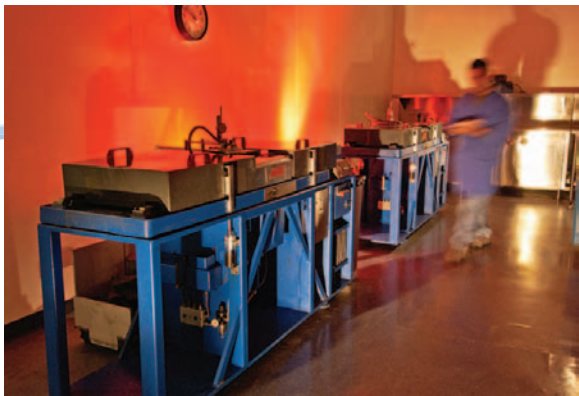
Quartz bars are lumbered, sliced and lapped. Wafers for special applications are further polished to an optical finish.
