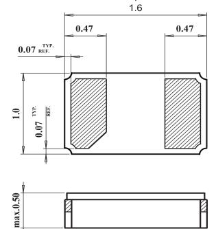
Package is Ceramic-Metal. Dimensions are millimeters.
