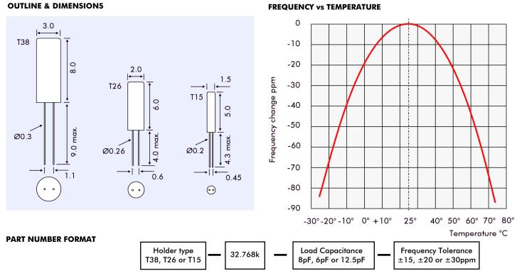
Example: T26-32.768k-6P-20 Represents: 2 x 6mm holder, 32.768kHz with CL = 6pF and tolerance ±20ppm
