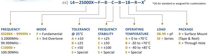
See below for legacy part numbering configuration for parts designed prior to 02-01-2014, which are still available
